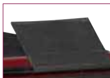
Rubber cover protects secondary controls
