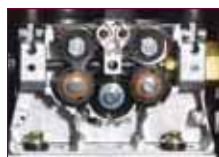
Heavy duty 4 roll precision drive system
