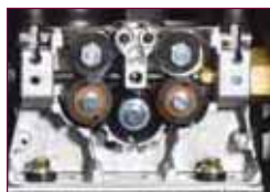
Heavy duty 4 roll precision drive system
